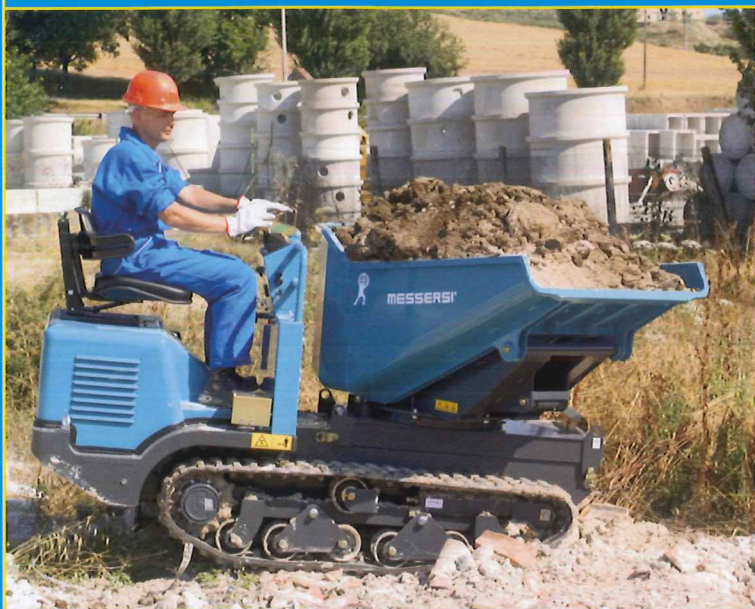
180° TCH-1500/BT swivelling skip during working phases / TCH-1500/BT mit 180° Drehmulde in Arbeitsphase / Бункер модели TCH-1500/BT вращается на 180°.
